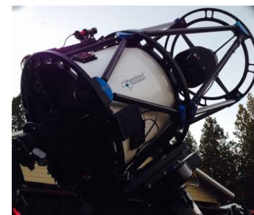
iTelescope.Net's 24 inch Planewave CDK
